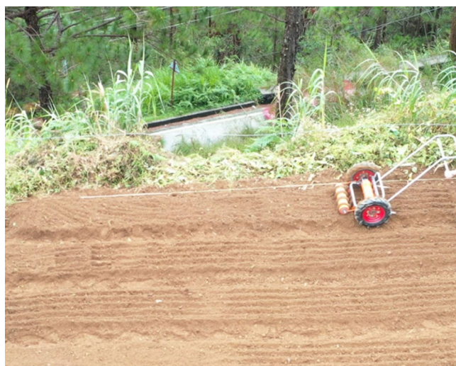
Figure 8. Field testing of the carrot seeder administered by the Agricultural Machinery and Testing Evaluation Center, University of the Philippines Los Baños (AMTEC-UPLB).
