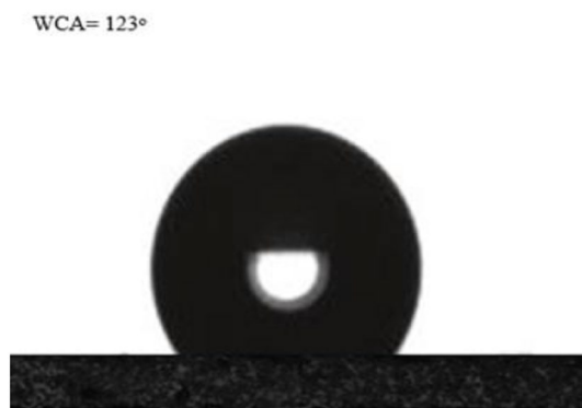
Figure 10. Water contact angle of PDMS/SiO 2 nanocoating on glass substrate.
