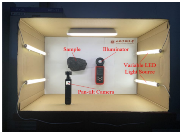
Figure 1. Multi-light source coal and gangue image acquisition system.
