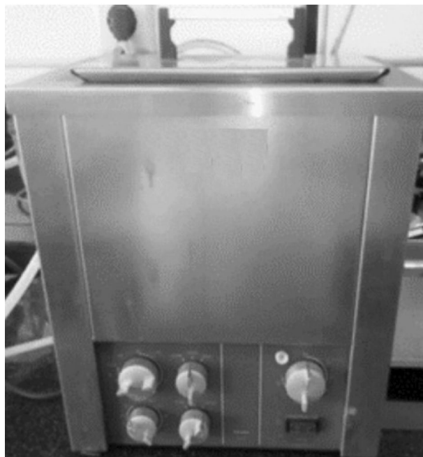
Figure 1. Photograph of bath sonicator used for the removal of DCF.
