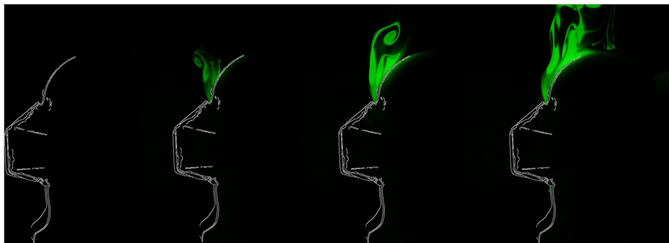
Figure 10. A sequence of four images taken automatically during an experiment a few seconds apart. DEHS aerosol is expelled from behind the mask. Illumination was provided by a 50 mW line laser module (wavelength 530 nm). All images had a still image subtracted from them to show only the aerosol and not the background. Additionally, a Canny edge detection filter was applied to better show the geometry of the head.
