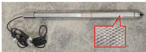
Figure 5. Rough pile (with the pile surface subjected to roughening (scoring) treatment).
