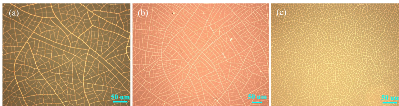
Figure 4. Optical microscope images of copper network films with different coating speeds: (a) 1500 r/min, (b) 2000 r/min, (c) 2400 r/min.
