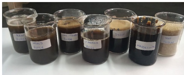
Figure 1. Major products obtained from the VHP sugar manufacturing process: raw juice, mixed juice, lime-treated juice, clarified juice, syrup, massecuite, and VHP sugar.
