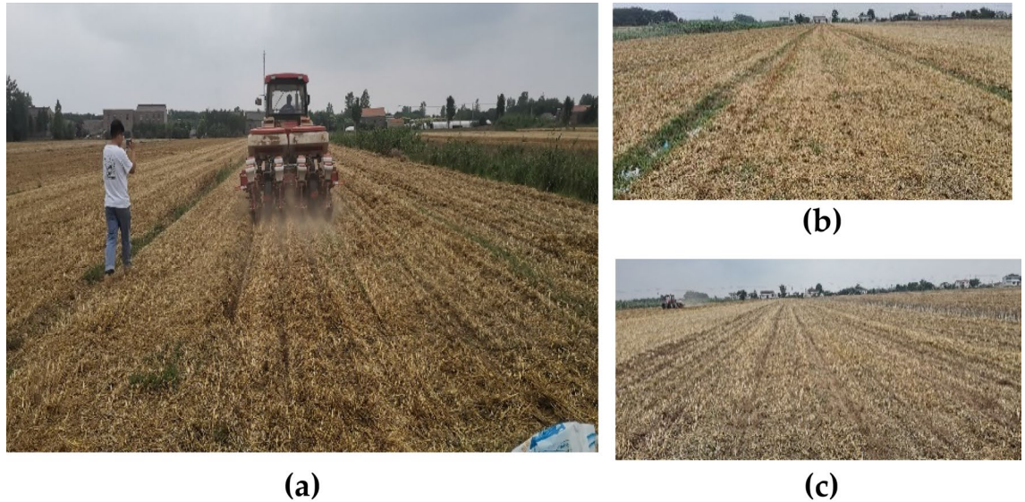
Figure 11. Field experiment under inclined seed-metering. (a) In-situ operation of the inclined seed-metering device; (b) field view before operation; (c) field condition after operation of the metering device.
