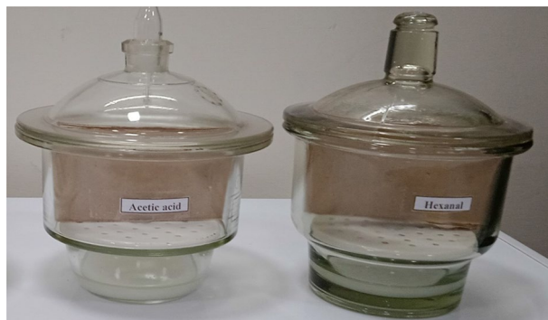
Figure 1. Paper exposed to VOCs in a desiccators.
