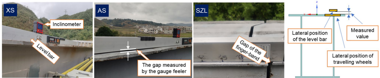
Figure 7. Configuration of the field tests to measure the LLI.
