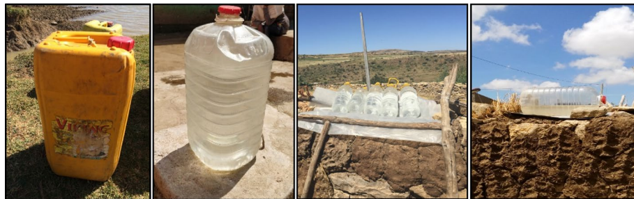
Figure 1. From left to right: Photographs of the standard opaque 25 L jerrycan used in Sub-Saharan Africa and 25 L PET TJC used for solar water disinfection and photographs of the 25 L PET TJC and 2 L PET bottles exposure on site in households of Tigray Region in Ethiopia.
