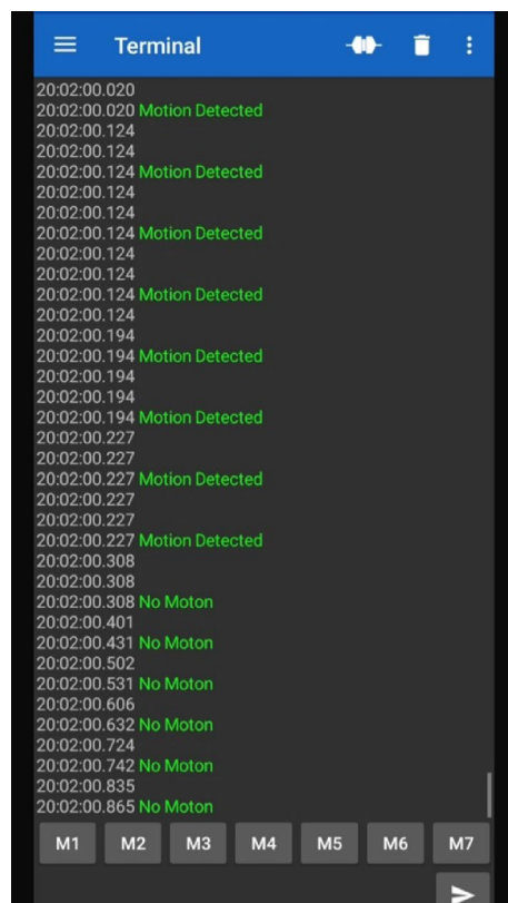
Figure 7. Motion Detection using ADXL 362 being visualized on a Bluetooth application.
