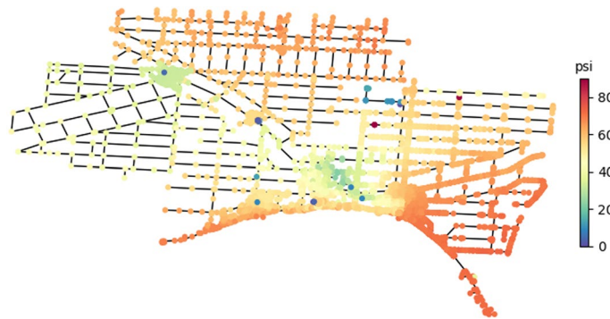
Figure 5. WDN pressure before the occurrence of earthquake and 48 h after the simulation started.
