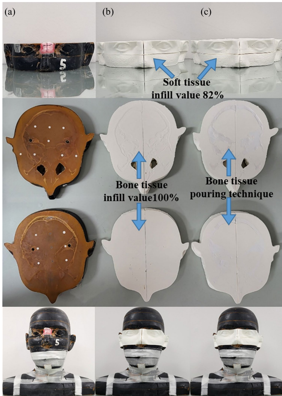
Figure 8. (a) Commercial Rando head phantom, (b) Rando head phantom printed using only PLA material, (c) Rando head phantom printed with a mixture of plaster and PLA powder.
