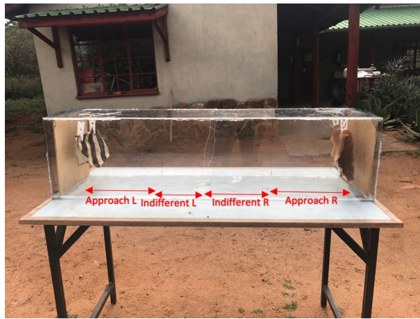
Figure 3. Experimental set-up for a plains zebra vs. impala skin trial. Landings were recorded as having occurred on a skin surface, within the approach zone of 30 cm from the skin, or in the indifferent zone of 30–60 cm from the skin on either side of the petri dish. Photo credit: LVR.
