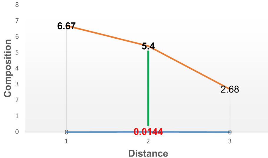
Figure 2. Diffusion of carbon atoms into the surface of grey cast iron at 900° for 60 min.
