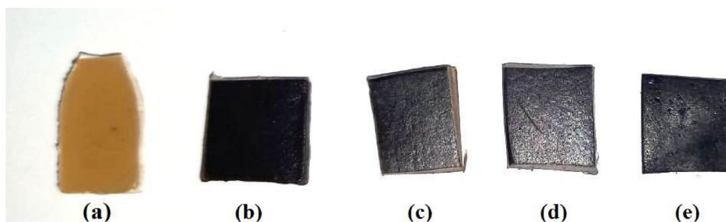
Figure 3. proposed amine-functionalized poly (vinylchloride/Linear low-density polyethylene)/ZnO with the selected different four amines; (a) ethylene diamine EDA, (c) aniline An, (d) p-anisidine pA, (e) N, N dimethyl aniline DMA and (b) a possible crosslinking mechanism for two products functionalized by diamine precursors. The photo in bottom is show the changing of samples color after amination reaction (a) (PVC/LLDPE)ZnO-b, (b) (PVC/LLDPE)ZnO-EDA, (c) (PVC/LLDPE)ZnO-An (d) (PVC/LLDPE)ZnO-pA and (e) (PVC/LLDPE) ZnO-DMA.
