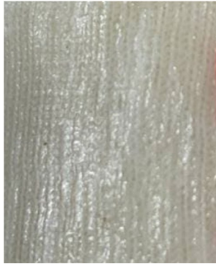
Figure 6. Internal surface of TF socket with 2:3 epoxy resin to hardener ratio.
