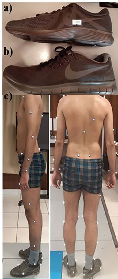
Figure 1. (a) Conventional running shoe, (b) auxetic Nike free RN shoe and (c) placement of Vicon markers in the sagittal and frontal planes.
