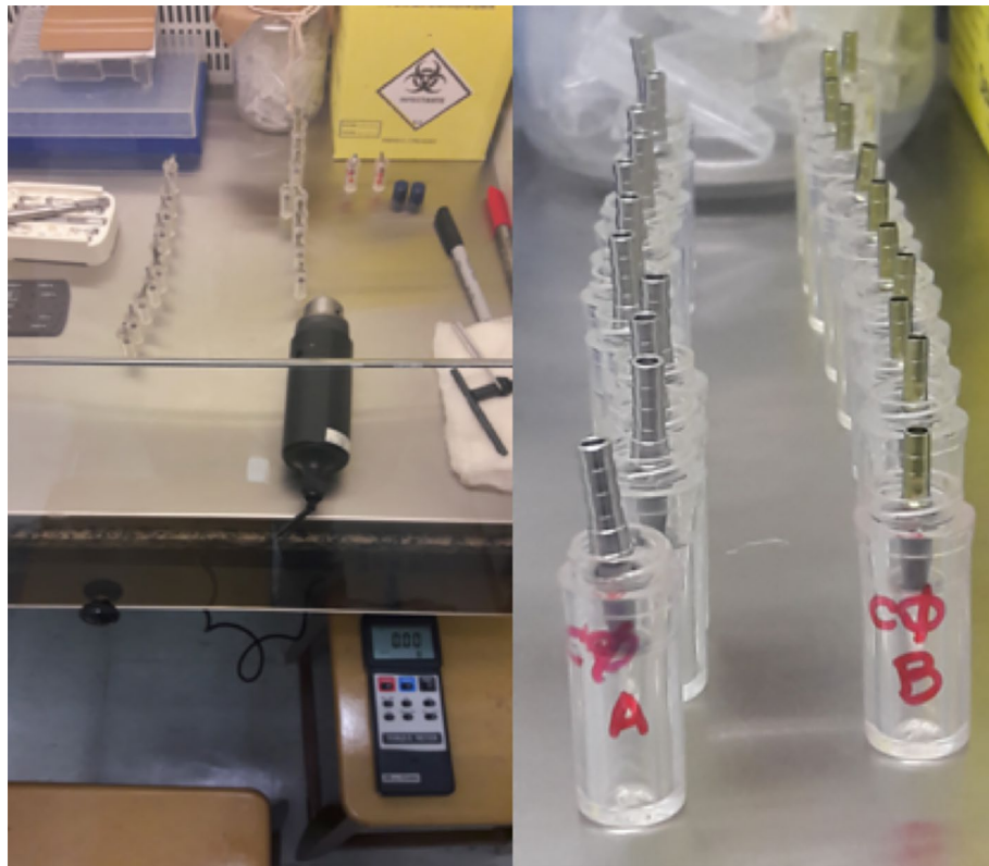
Figure 2. Sets of implants and abutments mounted in a laminar flow with aid of a digital torque wrench.
