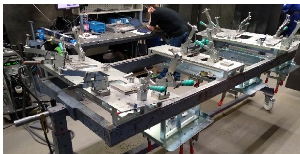
Figure 14. Welding jig for welding a door frame.
