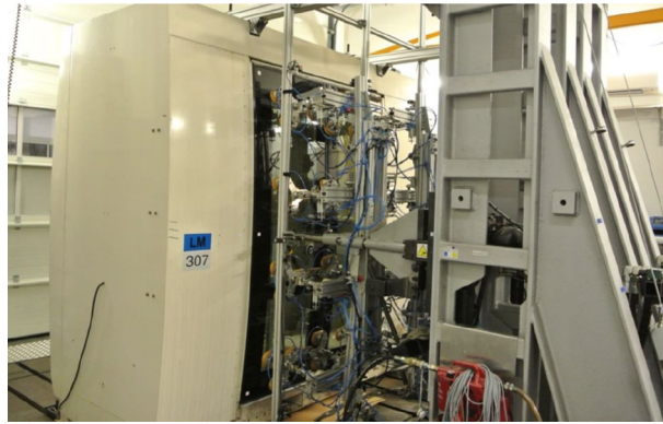
Figure 22. Real loading (dynamic) on the testing table.
