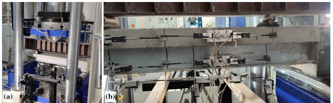
Figure 5. Examples of the bending test setup of the hybrid beam: (a) the surface exposed for digital image correlation; (b) distribution of linear variable displacement transducers, monitoring vertical and horizontal displacements.
