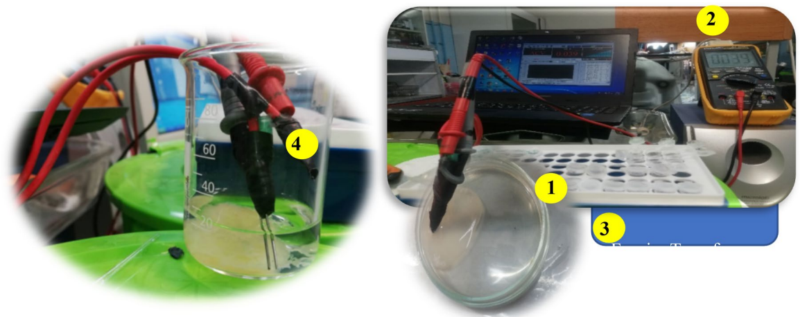
Figure 2. Adopted electrode system, implanted onto the cysts. (1) Petri dish containing cyst, (2) AVO meter, (3) DFFT algorithm and (4) Configuration of the adopted electrode system.
