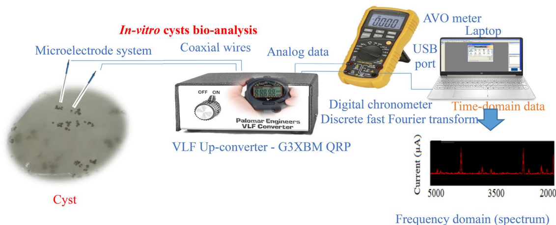
Figure 1. Schematic of the designed and introduced instrumentation system for cyst bio-analysis process.
