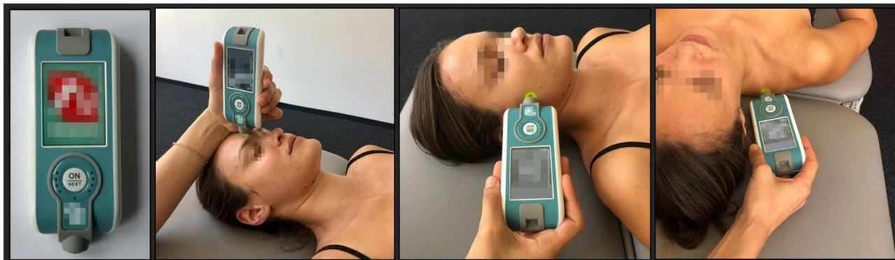
Figure 2. MyotonPRO; Legend: MyotonPRO and application for the CS, SM, and UT (from left to right).
