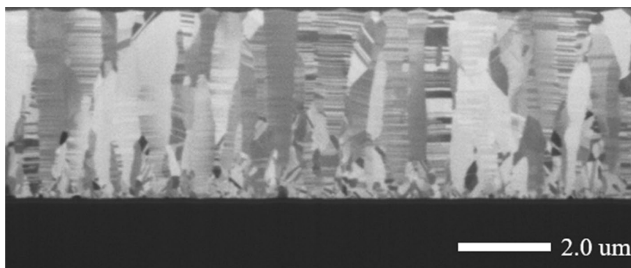
Figure 10. The FIB cross-sectional metallographs of the sputtered Cu films deposited with substrate bias of – 150 V on Si substrate.
