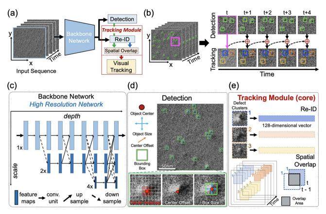
**Figure 3.** Overview of our *DefectTrack* model network. (a) *DefectTrack* architecture. (b) Schematics of how *DefectTrack* achieves tracking via detection and tracklets association. (c) The neural network architecture of the backbone network. (d) *DefectTrack's* detection branch. (e) *DefectTrack's* core tracking module.
