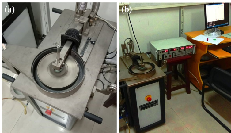
Figure 10. Wear test (a) sliding disc, (b) pin on disc setup.
