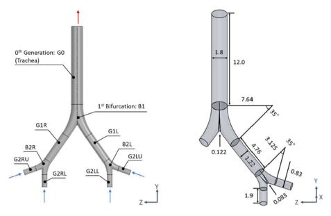
Figure 2. Airway model: (left) name of each part; (right) diameter, length, and angle.
