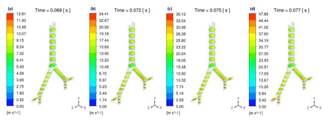
Figure 3. Velocity contours for cross-sections of the airway at PVT.
