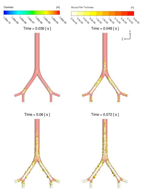
Figure 6. Generated droplets and thickness of the mucous film over time at CPFR=4 L/s.
