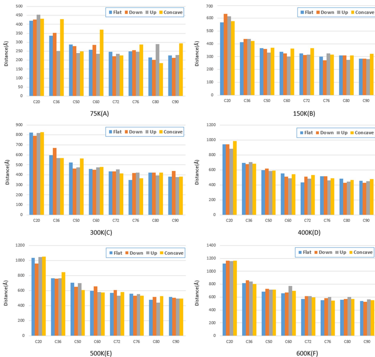
Figure 9. Traveled distance by fullerenes on a gold substrate for 75K (A), 150K (B), 300K (C), 400K (D), 500K (E), and 600K (F). The blue, red, black and yellow bars show the traveled distance of the molecules on the flat, down side of the step, top side of the step, and concave substrates, respectively.
