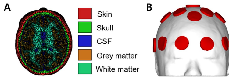
Figure 2. The model used for FEM calculation. (A) MRI-based realistic finite element model; consists of the skin, skull, cerebrospinal fluid, gray matter, and white matter, (B) scalp surface with circular electrodes with an area of 8 cm 2 generated.
