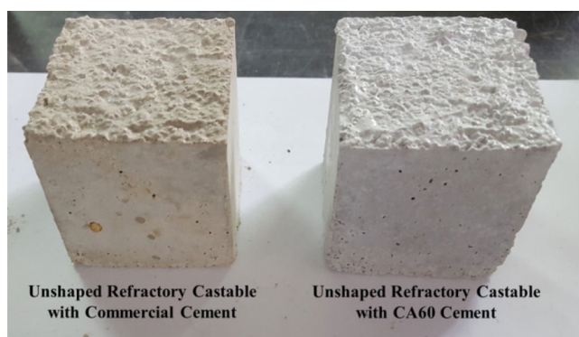
Figure 12. Unshaped refractory castables using CA60 sintered at 1450 °C and commercial cement.
