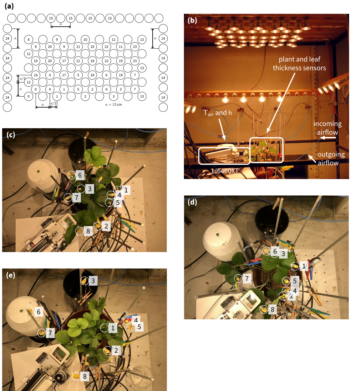
Figure 5. Overview of the three experiments and leaf thickness sensor locations. The clip number of each sensor is depicted in the figure. (a) Lamp grid on the top and sides of the frame. Circles indicate a single LED lamp and the numbers indicate the group to which this lamp belongs. Empty sockets are circles without a number. The left, right and top rows (groups 24, 14 and 15 respectively) were mounted on the sides and help to create directional lighting. (b) Entire setup inside the growth chamber. Different measurement instruments are indicated as well as the airflow inside the growth chamber. (c)–(e) Images depicting the setup at the end of each experiment: (c) strawberry 1, (d) strawberry 2 and (e) the control experiment. Carefully observe that the clips are not mounted on the plant in (e). There are also two unlabelled clips visible in the images, these were discarded due to sensor failure.
