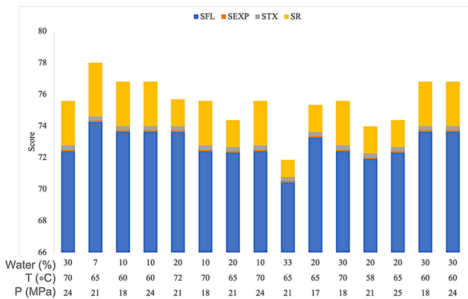
Figure 5. Individual factors in the CSTS score at each parameter for the SFE of G. procumbens .
