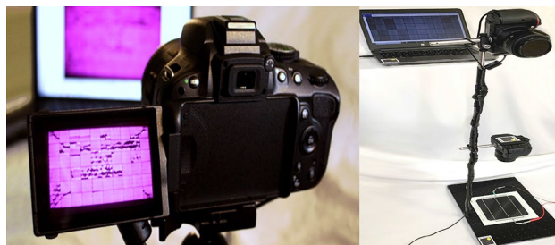
Figure 2. EL imaging setup.
