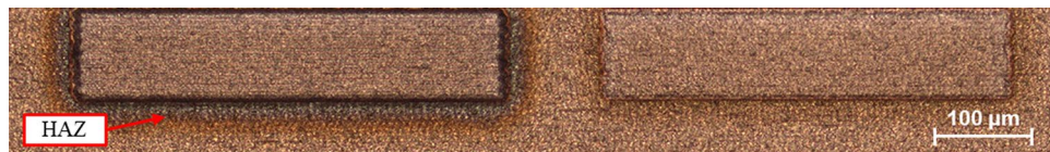
Figure 12. Comparison of laser processing of copper without gas processing (left) and with gas processing (right).
