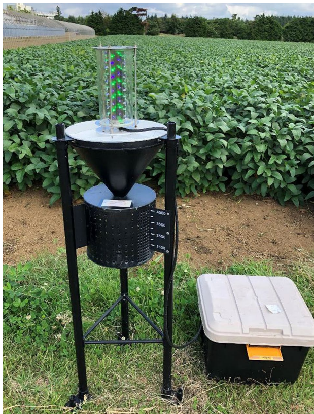
Figure 4. Photograph of combined UV and green LED trap used in the experiments.
