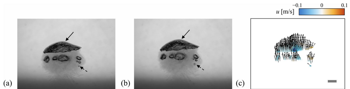
Figure 11. (a,b) Consecutive images (with a time separation of 2.5 ms) of the cap bubble and a few smaller bubbles. (c) Corresponding velocity field obtained by the fine-tuned CNN-based optical flow (the contour denotes the horizontal velocity). The solid bar in (c) denotes 10 mm.
