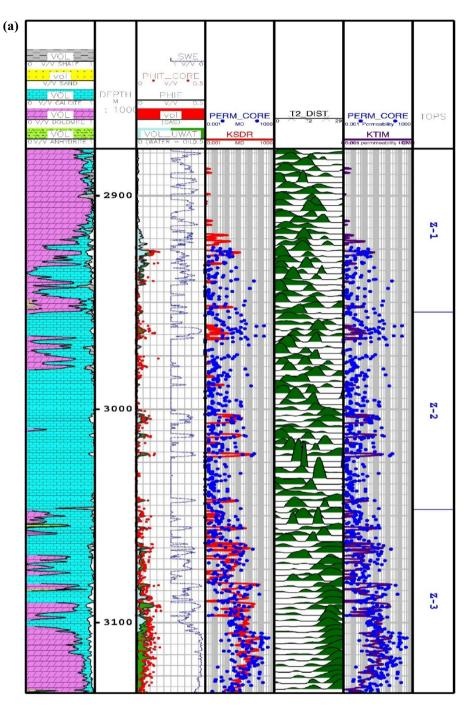
**Figure 6.** Comparison of the permeability derived from NMR logs with the core permeability data: (**a**) from Asmari zone 1 to zone 3; (**b**) from Asmari zone 4 to top of PD formation (PD: Pabdeh formation; T2\_DIST: distribution of T2 relaxation time; KSDR: SDR permeability; KTIM: Timur permeability).
