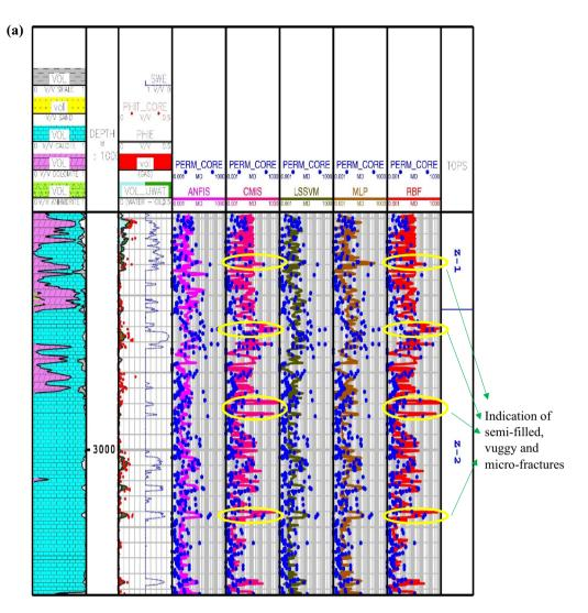
**Figure 5.** Comparison of the permeability derived from smart mathematical strategy with the core permeability data: (**a**) from Asmari zone 1 to zone 2; (**b**) from Asmari zone 3 to zone 4; (**c**) from Asmari zone 5 to top of PD formation (SWE: effective water saturation; PHIE: effective porosity; PHIT\_CORE: core permeability; TOPS: tops of geological zonation; PD: Pabdeh formation; VOL: volumetric composition of each mineral).
