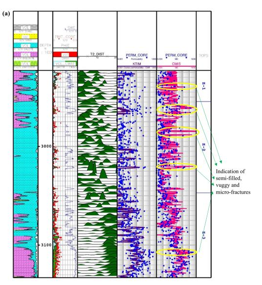
**Figure 7.** Comparison of the CMIS smart strategy developed in this study with Timur-Coates NMR model: (a) from Asmari zone 1 to zone 3; (b) from Asmari zone 4 to top of PD formation.
