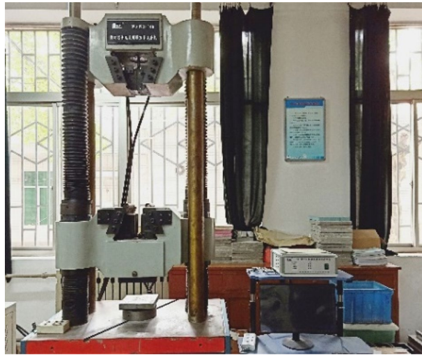
Figure 3. The WAW31000 microcomputer control universal testing machine.
