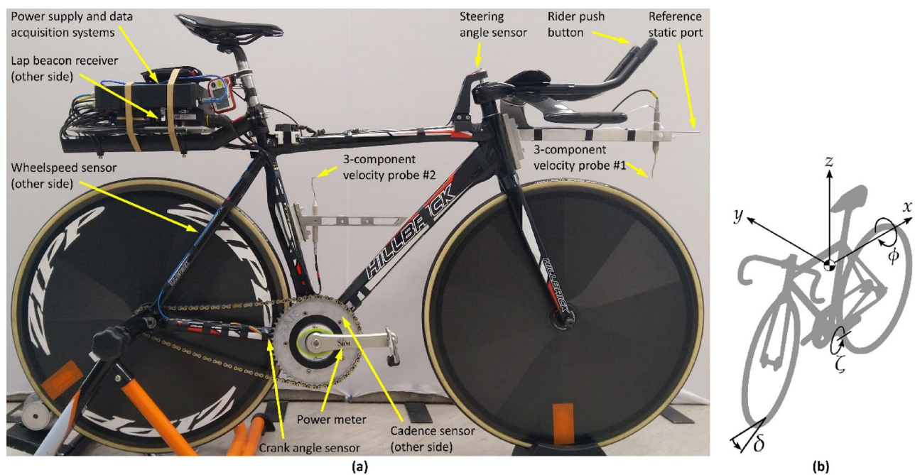
Figure 1. (a) Primary bicycle used for testing and (b) bicycle coordinate system.
