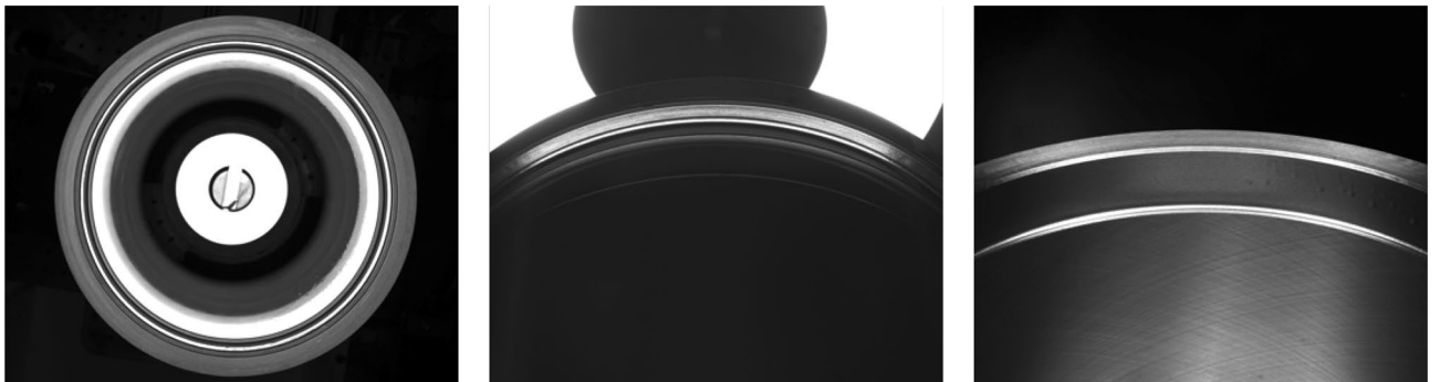
Figure 3. Three cylinder liner examples taken by an area-array CCD camera.
