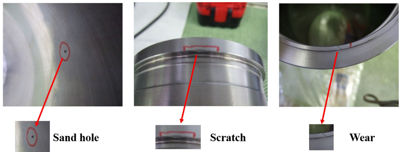
Figure 1. Three frequently occurring cylinder liner defects. The images from left to right represent sand hole, scratches, and wear, respectively.
