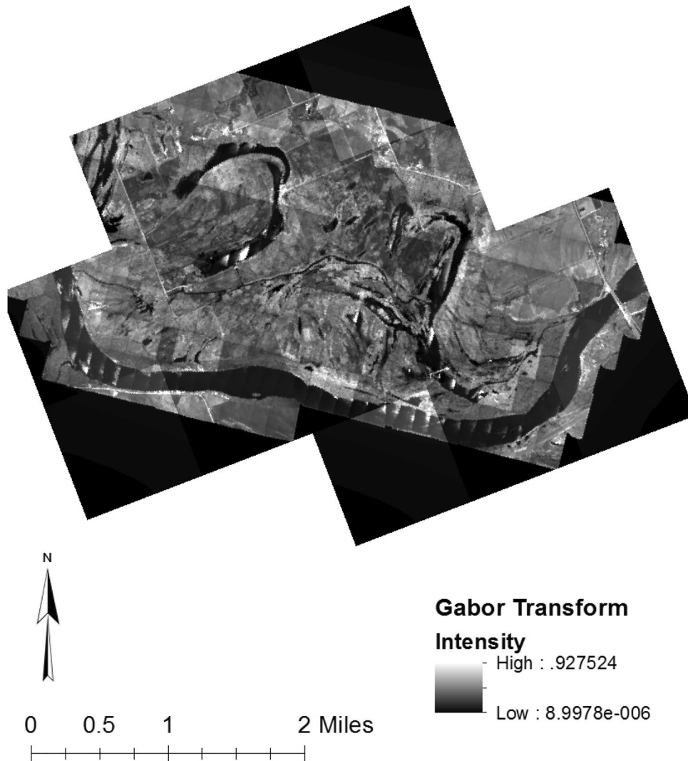
Figure 2. Gabor transformation. Gabor transformed image of study area derived from original image using the first principal component of all gabor outputs using the filter bank parameters. Software: ArcMap (10.x).
