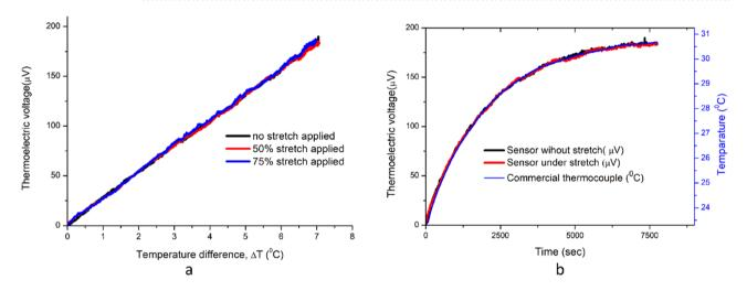
**Figure 7.** The temperature sensing using proposed sensor at different strain conditions (**a**) Temperature rise at the hot junction over time monitored with the sensor in unstretched and stretched (50% strain) conditions. Simultaneously, the hot junction temperature measurement with a commercial thermocouple (**b**).
