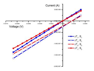
**Figure 8.** Simultaneous measurement of temperature and strain.  $\Delta T1$ ,  $\Delta T2$  indicates two different temperature differences and S indicates the strain. The slope of the graph gives the strain-caused resistance change of the device, while the temperature-generated voltage can be read from the voltage shift on the horizontal axis.
