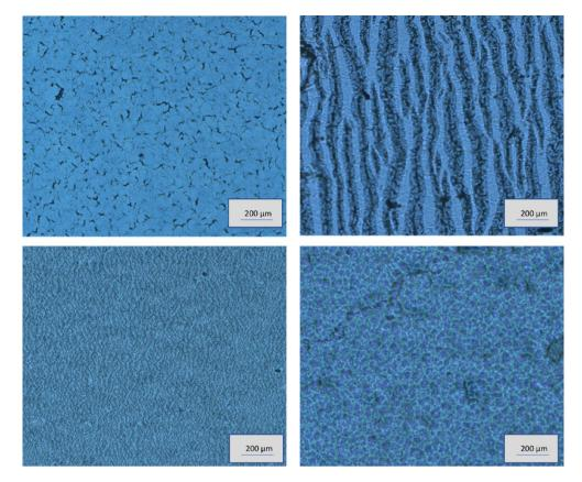
**Figure 3.** Microscopic images of PEDOT:PSS layers with varying proportions of stretching enhancers kept for stretching. Layer morphology of PEDOT:PSS composition with no addition of stretchability enhancers (**a**), after stretching it to 100% strain value (**b**), the resultant layer of PEDOT:PSS with stretchability enhancer of 5wt% and 15wt% respectively at 100% strain condition (**c**, **d**).
