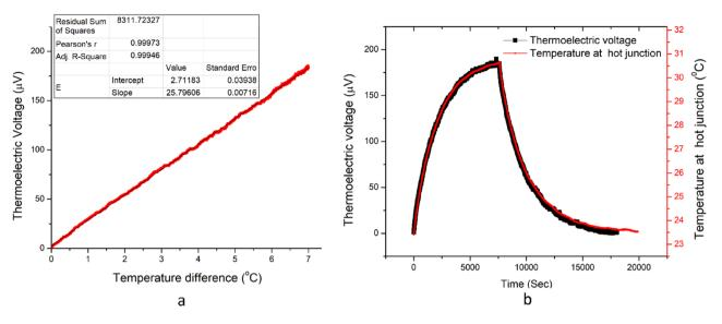
**Figure 6.** Temperature induced thermoelectric voltage in the sensor is plotted (**a**), Sensor applied for measuring the heating and cooling of heater coil shown with the proposed sensor and commercial thermocouple (**b**).
