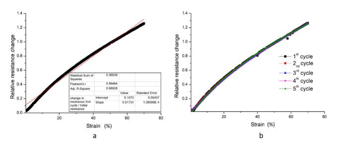
**Figure 4.** Normalised resistance change of the sensor for 70% strain (**a**) and demonstration of reproducibility of the sensor measurements (**b**).
