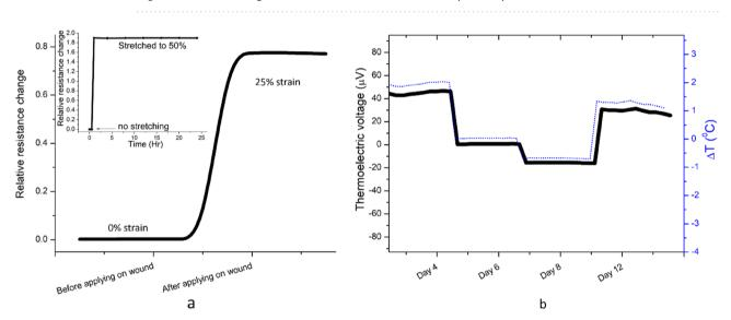
**Figure 10.** Strain induced resistance change upon applying the sensor on mice body (**a**), sensor resistance change is measured while it is elongated to 50% using a stretch bench and maintained it in the same position for 24 h (**a**, insets). Thermoelectric voltage generated during the test period of 4–12 days and corresponding  $\Delta T$  is also shown in **b**.
