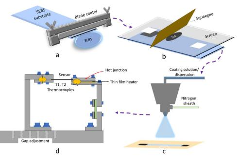
**Figure 1.** SEBS substrate preparation with blade coating (**a**); Screen printing silver electrodes on SEBS (**b**); Spray coating PEDOT:PSS based composition on SEBS substrate which is selectively masked (**c**); Temperature sensor characterisation set up (**d**).
