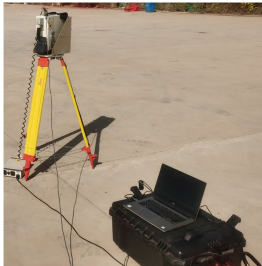
Figure 7. The experimental site was chosen to be in a flat and open area, and the HPGe γ spectrometer was set up at the height of 1 m from the ground and connected to a computer. Place the radioactive sources in sequence according to the grid division method described in Fig. 6 to complete the experiment.
