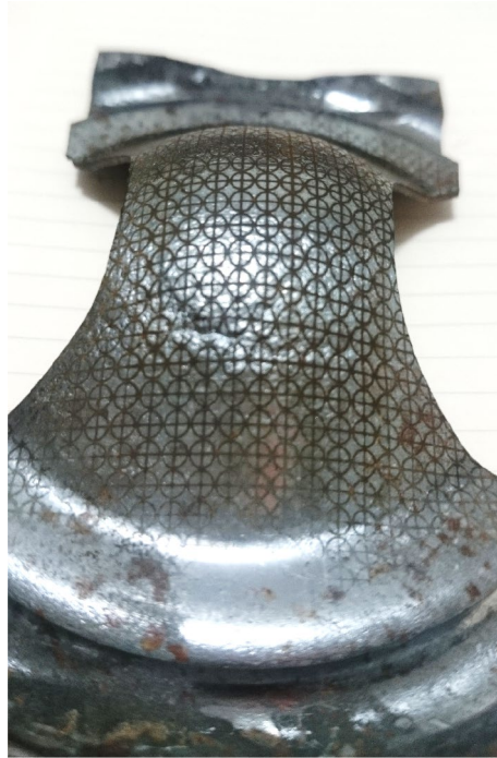
Figure 6. Forming limit sheet samples after Nakazima's punch test.
