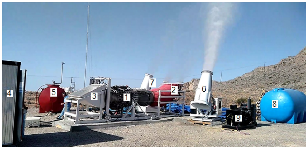
Figure 6. Experimental complex in operation: (1) aircraft engine D-30; (2) nozzle for directing the jet up; (3) engine air receiver; (4) engine start and control cabinet; (5) jet fuel tank; (6) Fog Cannon JY-60; (7) Fog Cannon WP-60; (8) tank for hygroscopic substances solutions; (9) diesel generator 3 × 380 50 kW to feed the Fog Cannon JY-60.
