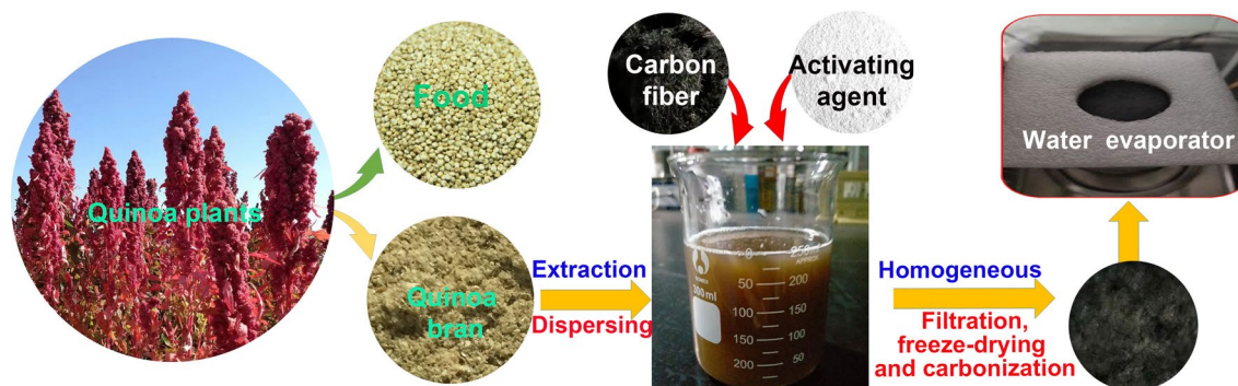
Figure 1. Schematic exhibition for the fabrication steps of CFQC based evaporators. Farmland site is located in Jingle County, Xinzhou City, Shanxi Province, China. Quinoa plants is photographed by Jie Yang, Department of Chemistry of Xinzhou Teachers University.
