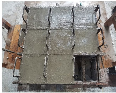
Figure 1. Mold used for preparation of fractured specimens of soft rock-like material.
