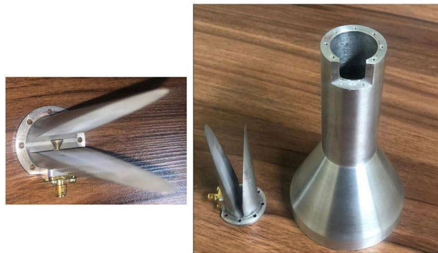
Figure 12. Fabricated horn antenna along with its wideband coaxial to waveguide transition.
